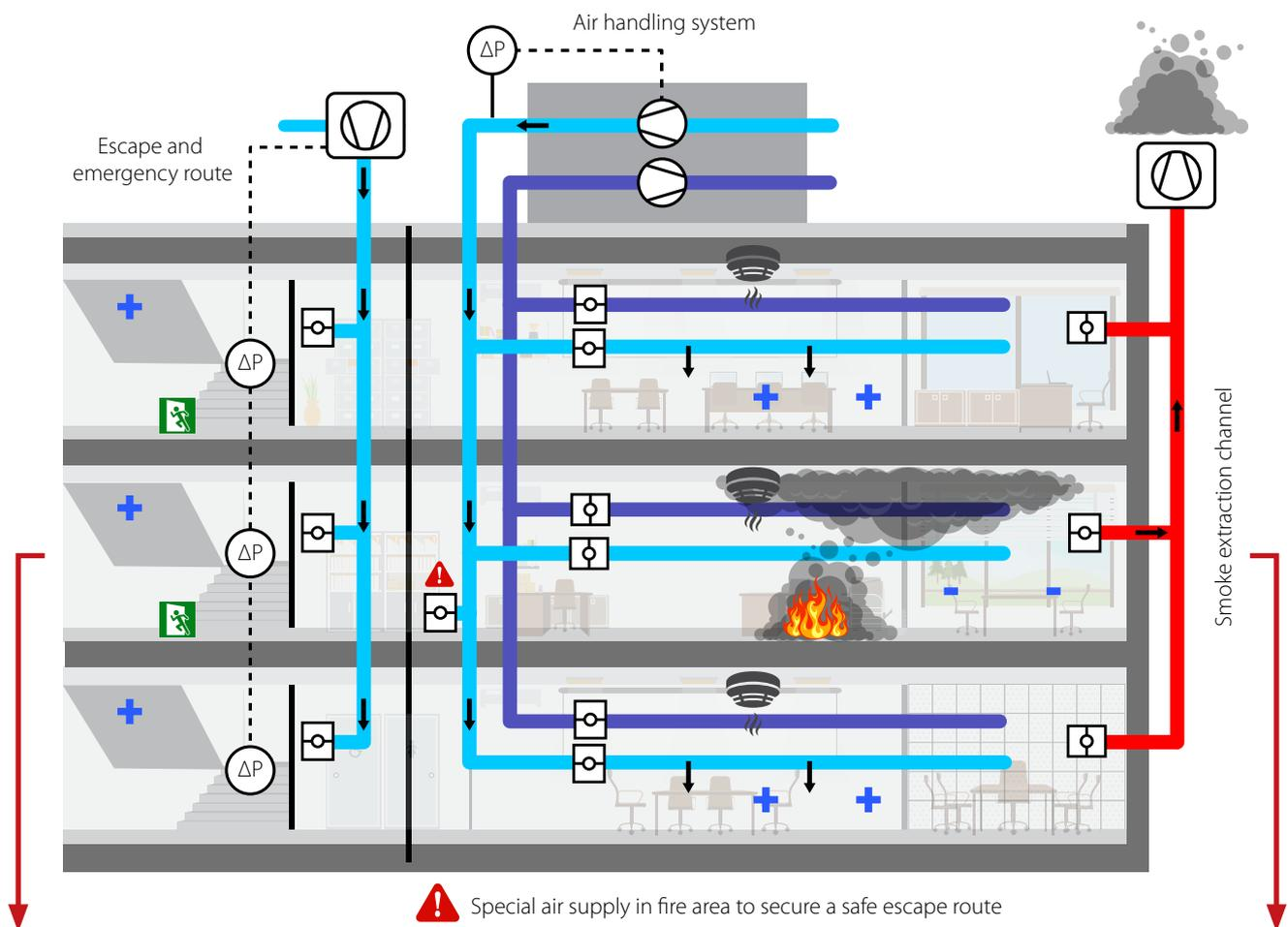
**The stairwell overpressure system** prevents smoke entering the escape area. The maximum overpressure is limited to a level that ensures personnel can still open the doors and enter the stairwell.
