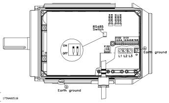
The control cables must be screened cables
