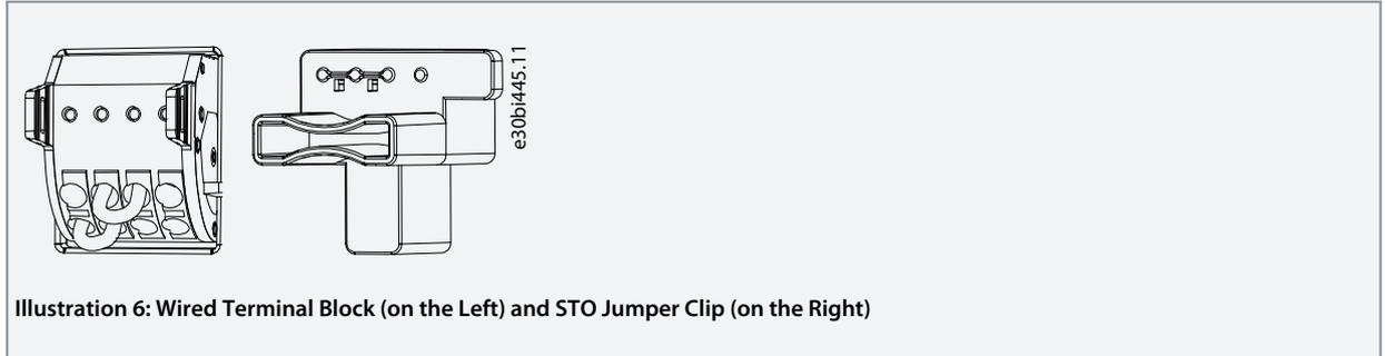
Illustration 6: Wired Terminal Block (on the Left) and STO Jumper Clip (on the Right)
