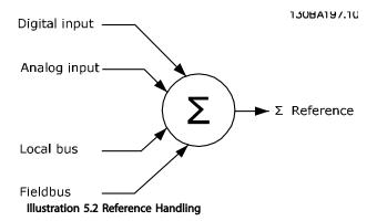
The reference, or speed set point (MRV, sent via POWERLINK), is always transmitted to the frequency converter in percentage format as integers represented in hexadecimal (0-4000 hex).
