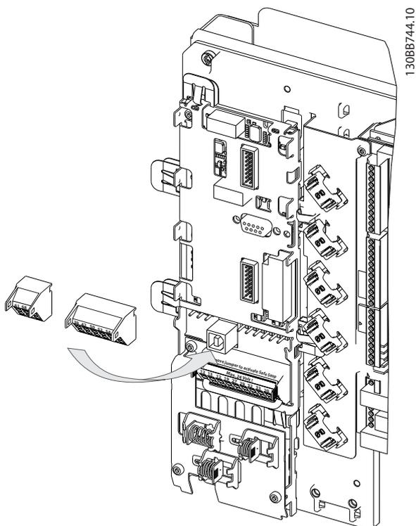
AC line (jumpers between 100-102 and 101-103). If external supply is needed, the jumpers are removed and the supply is connected to terminals 100 and 101. A 5 Amp fuse should be used for protection. In UL applications this should be LittleFuse KLK-5 or equivalent.
