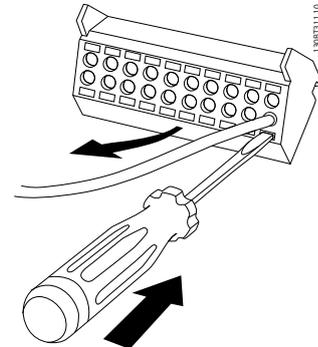
4. Remove the screwdriver. The cable is now mounted in the terminal.
