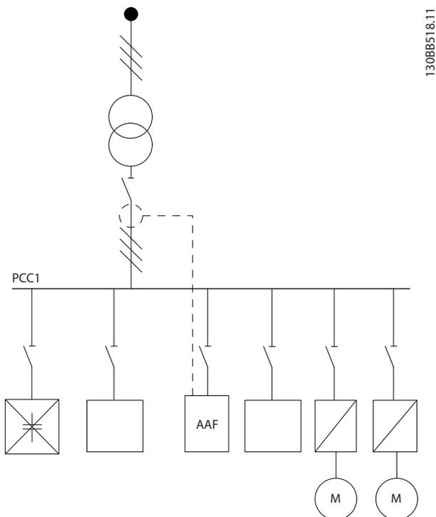
**Illustration 4.37** Not allowed installation. Corrected capacitor current interacts with CT measurement.
