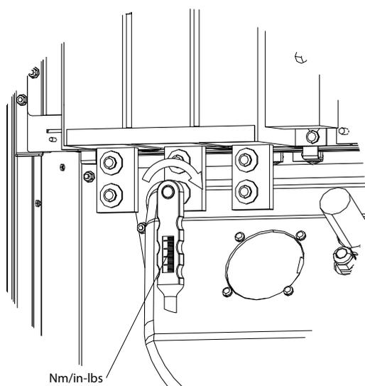
Illustration 4.28 Tightening Bolts with Torque Wrench
