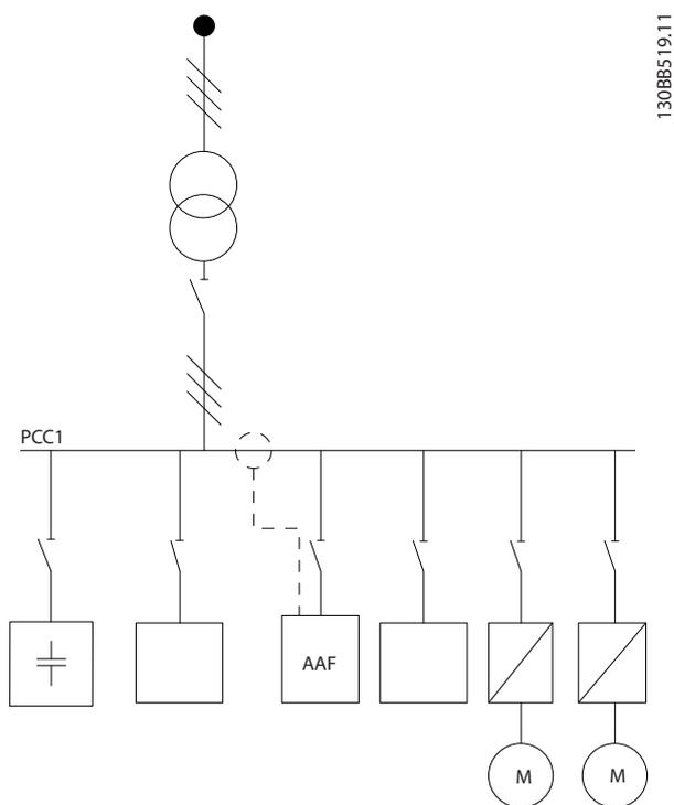
**Illustration 4.38** CT's installation does not measure capacitor current.
