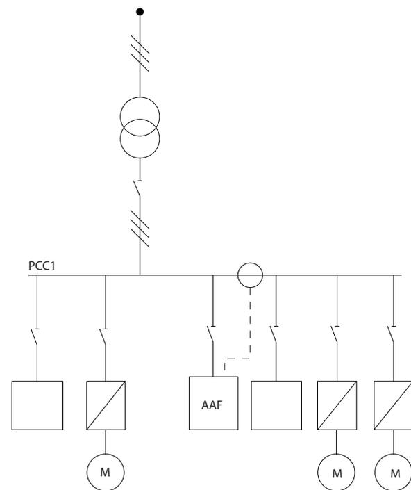
Illustration 4.33 Current transformers installed on load side for group compensation.
