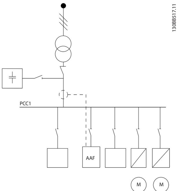
**Illustration 4.36** Capacitor bank mounted up stream and CTs installation does not measure capacitor current.
