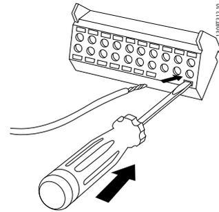
3. Insert the cable in the adjacent circular hole.
