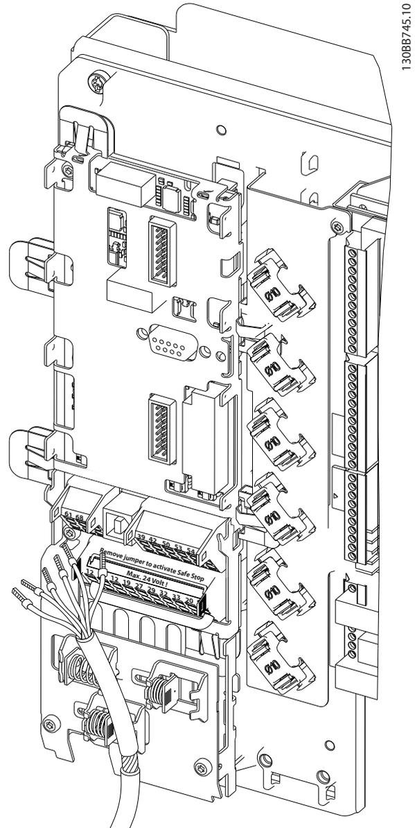
Remember to connect the shields in a proper way to ensure optimum electrical immunity.
