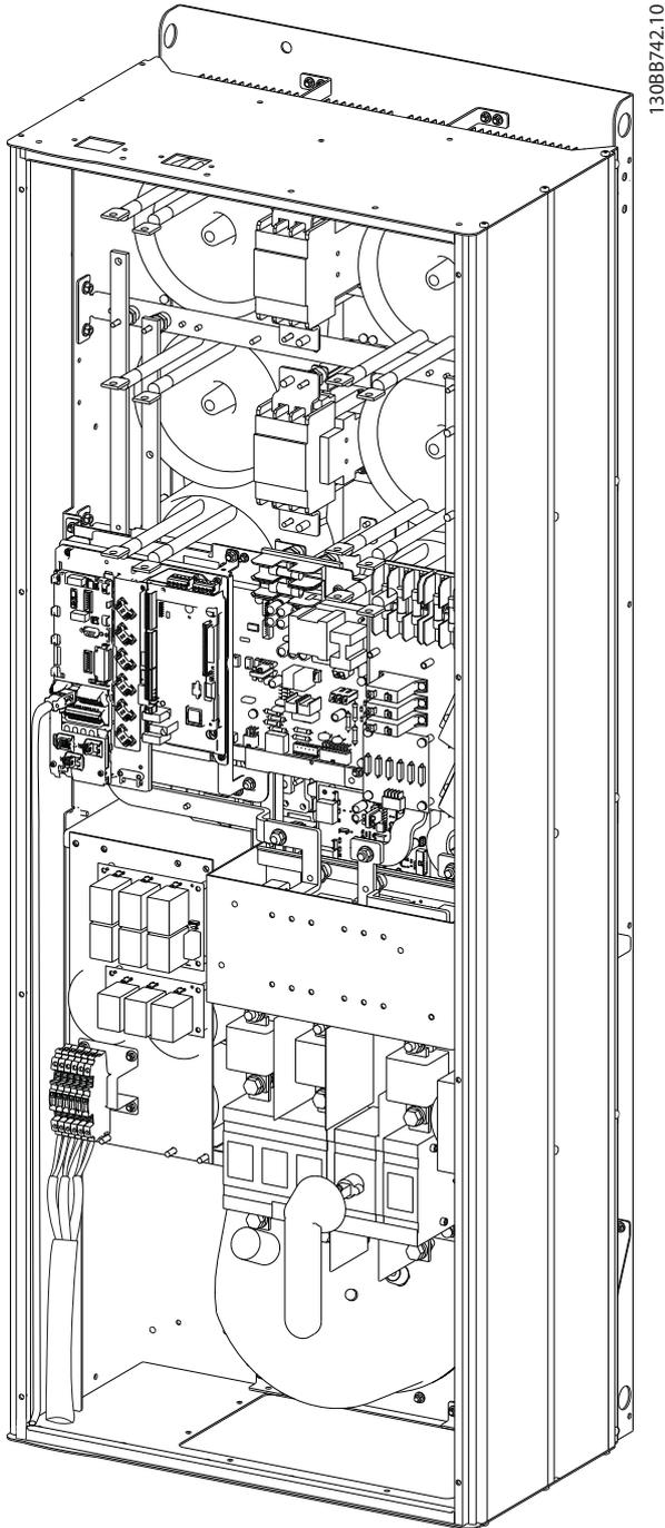
Illustration 4.40 Example of Control Card Wiring Path, D13.
