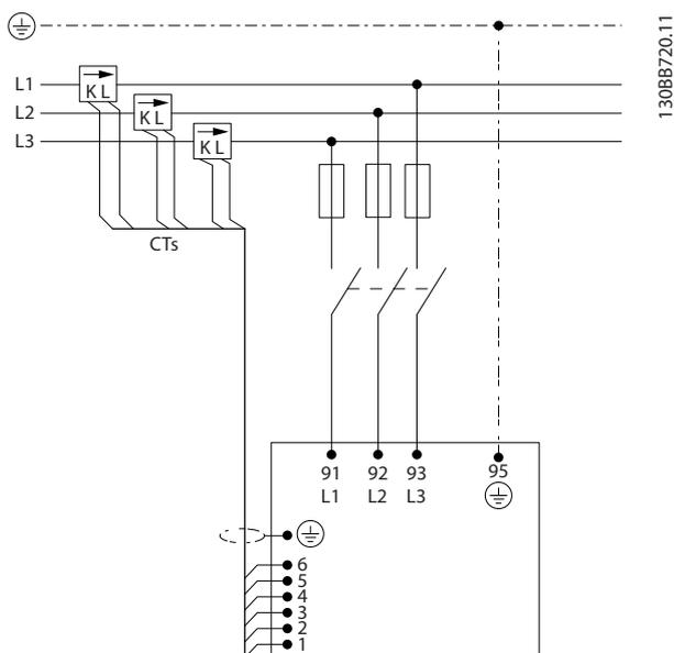
Illustration 4.1 Diagram showing basic installation including mains and CTs.
