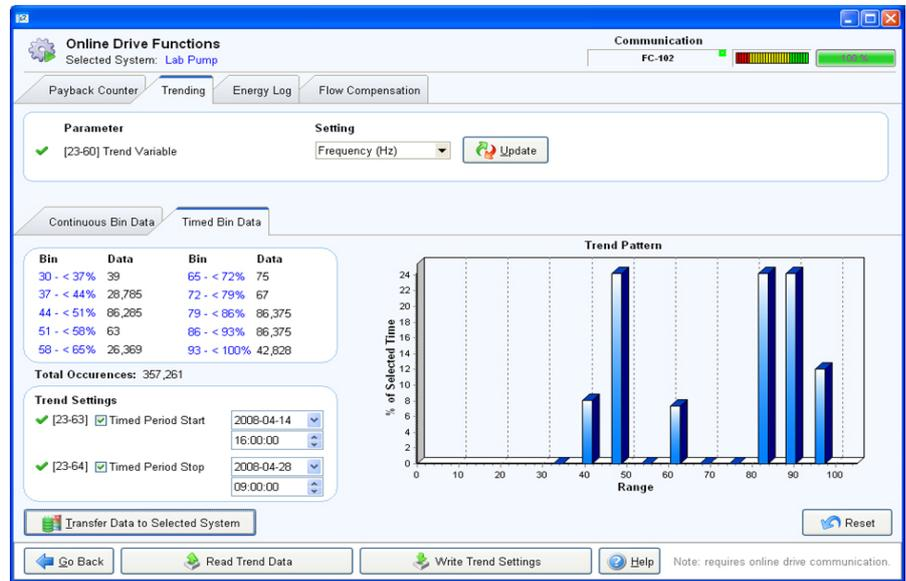
Bin data representing the system speed (Hz or RPM) is converted into a load profile or duty cycle by the
