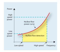
No flow based on motor power and frequency
