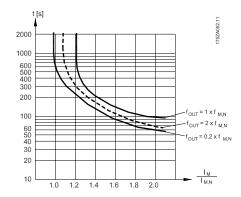
The ETR feature is calculating the motor temperature based on actual current and speed. The calculated temperature is visible as a read out parameter in P16-18 in the FC202.
