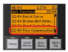
The drive software makes programming the Flow Compensation feature quick and easy by choosing Application Functions Group 22, under the Main Menu and selecting 22-8\* Flow Compensation. The VLT® HVAC Drive provides a special flow compensation feature for pump systems to reduce energy consumption. This feature is useful when it is not possible for a pressure transducer to be placed at the most distant significant load in the system and it can only be located close to the pump.
