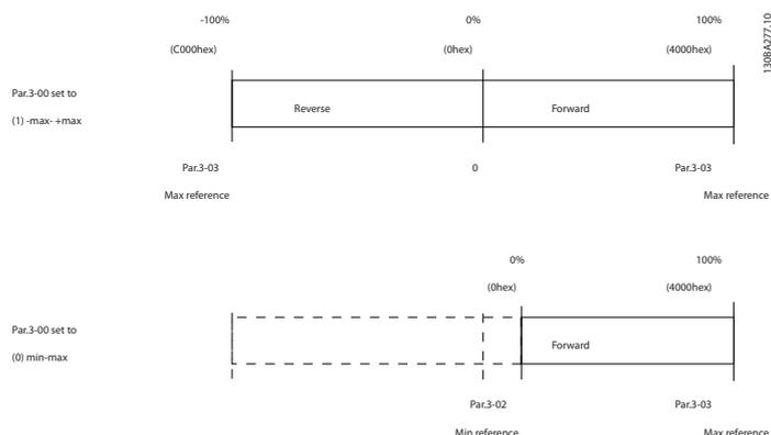
The actual reference [Ref. %] in the frequency converter depends on the settings in the following parameters:
