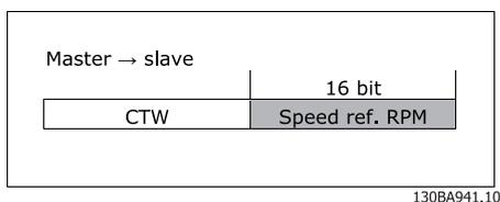
The speed reference value should be transmitted to the frequency converter in the form of a 16-bit word. The value is transmitted directly in RPM.
