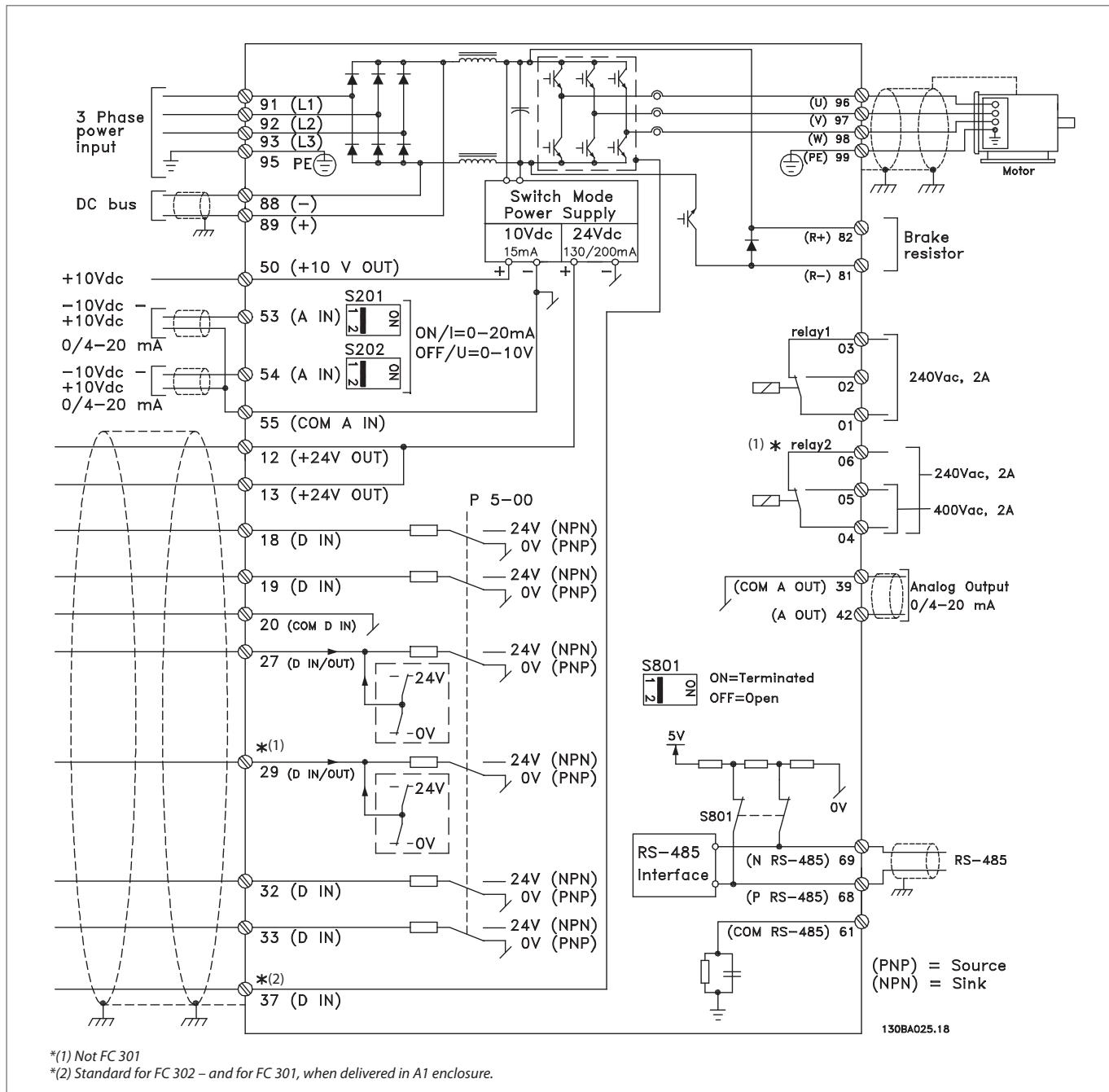
The diagram shows the port terminals of the FC 301 and FC 302. Additional options will expand the number of terminals.
