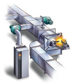
Advanced broken belt detection is based on motor torque. Torque is a better indication of a no-load condition because it avoids the need to compensate for motors with poor power factor (high current) at low load.
